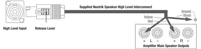
• For Differential (i.e. fully balanced) amplifiers using one REL, simply use the standard connecting scheme above. Connect the black wire to a ground lug or chassis screw. Should hum occur using this method, the black wire should be allowed to "float" or hang down without connection to ANY terminal.
