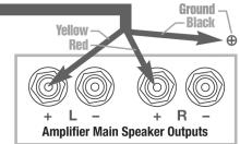
NOTE: Serie T/x models are equipped with internal circuitry to allow connection to many Class D (digital) amplifiers
