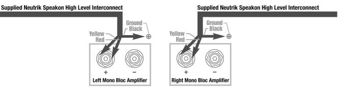
• If connecting a single REL as a dedicated centre channel sub, an insider tip is to consider connecting to the rear of the speaker, rather than routing the REL High Level enable all the way back to the amplifier. Connect the black wire of the REL to the negative centre channel speaker terminal; twist together the red and yellow wires and connect this paired cable (red/yellow paired together) to the positive centre channel speaker terminal.
