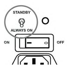
During initial setup, use the REL this way. After initial setup, if you wish to employ the standby mode, simply move the power mode switch into the up position to "STANDBY".
