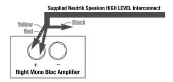
• If connecting a single REL as a dedicated center channel sub, connect the black wire of the REL to the negative center channel speaker terminal; twist together the red and yellow wires and connect this pair to the positive center channel speaker terminal.
