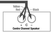
• If connecting a REL as a dedicated rear channel sub, connect the black wire of the REL to either the left rear or right rear negative speaker terminal; connect the yellow wire to the left rear positive speaker terminal; connect the red wire to the right rear positive speaker terminal. If the amplifier is of balanced differential design, please follow the instruction in the section above labeled Differential Connection.
