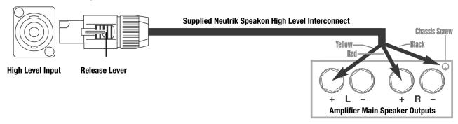
**NOTE:** The REL AirShip II transmitter is equipped with internal circuitry to allow seamless connection to Class-D (digital) main amplifiers. If connecting to a Class-D amplifier, follow the above connection procedure for differential amplifiers.
