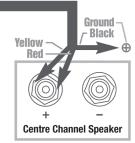
• If connecting a REL as a dedicated rear channel sub, connect the yellow wire to the left rear positive speaker terminal; connect the red wire to the right rear positive speaker terminal, connect the black wire to a ground lug or chassis screw. If the amplifier is of balanced differential design, please follow the instructions in the section above labeled Differential Connection.
