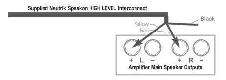
**NOTE:** The TZERO MKIII is equipped with internal circuitry to allow seamless connection to Class-D (digital) main amplifiers. If connecting to a Class-D amplifier, follow the above connection procedure for differential amplifiers.
