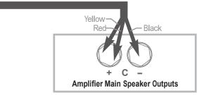
• If connecting a REL as a dedicated rear channel sub, connect the black wire of the REL to either the left rear or right rear negative speaker terminal; connect the yellow wire to the left rear positive speaker terminal; connect the red wire to the right rear positive speaker terminal. If the amplifier is of balanced differential design, please follow the instructions in the section above labeled Differential Connection.
