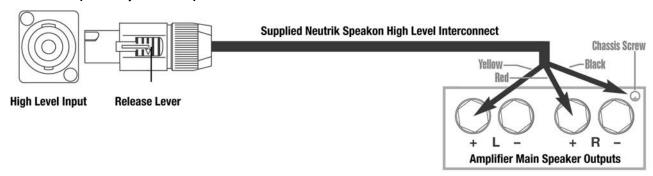
**NOTE:** The REL AirShip<sup>m</sup> transmitter is equipped with internal circuitry to allow seamless connection to Class-D (digital) main amplifiers. If connecting to a Class-D amplifier, follow the above connection procedure for differential amplifiers.
