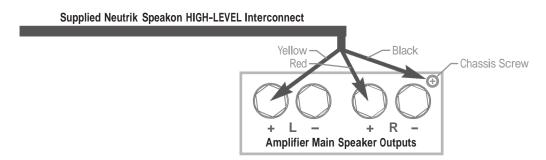
**NOTE:** The Tzero is equipped with internal circuitry to allow seamless connection to Class-D (digital) main amplifiers. If connecting to a Class-D amplifier, follow the above connection procedure for differential amplifiers.
