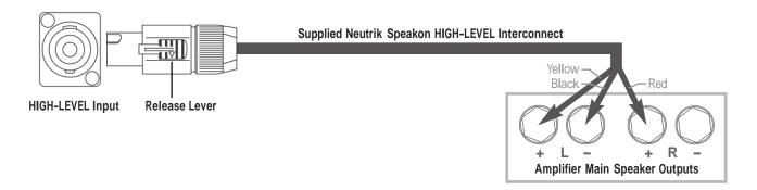
• For differential (i.e. fully balanced) amplifiers using one REL, simply use the standard connecting scheme with the exception of connecting the black wire to chassis ground (i.e. a metal bolt or screw, preferably not painted or anodized, on the chassis of the power amp or receiver), not to a negative speaker terminal, and then connecting into the HIGH-LEVEL input on the REL. Please contact your dealer should there be any questions concerning this or any other hookup procedure.
