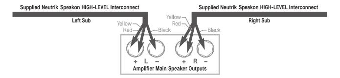
• If connecting a single REL as a dedicated center channel sub, connect the black wire of the REL to the negative center channel speaker terminal; twist together the red and yellow wires and connect this pair to the positive center channel speaker terminal.
