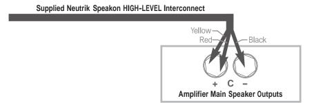
• If connecting a REL as a dedicated rear channel sub, connect the black wire of the REL to either the left rear or right rear negative speaker terminal; connect the yellow wire to the left rear positive speaker terminal; connect the red wire to the right rear positive speaker terminal.
